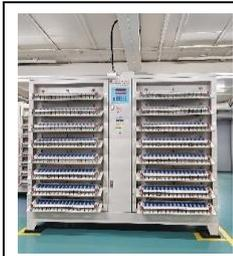
The Battery Formation and Grouping System is an important process in the production and quality assurance of lithium batteries. This system ensures that each battery cell meets specific performance and safety standards before being assembled into battery packs.
