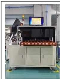
Cell grading process is performed using a Cell Sorting Machine, which automates the grading and sorting of battery cells based on various performance metrics like Capacity, Voltage, Internal Resistance etc. The purpose of cell grading is to ensure only high-quality cells are used in battery packs, reducing the likelihood of defects and failures and to identify and discard cells that do not meet safety standards, thereby preventing potential hazards like short-circuiting.
