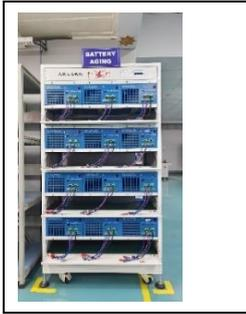
The Battery Testing System device plays a vital role in the testing the capacity, cycle life, performance, safety, internal resistance of the battery pack
