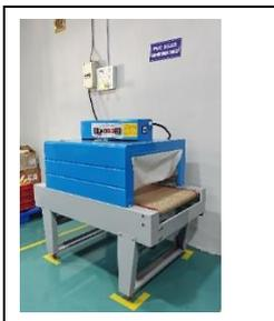
Sleeving involves enclosing the battery pack in a protective sleeve made of PVC. This process ensures the battery pack is insulated, protected from physical as well as environmental damage, and maintained in a compact and safe form.
