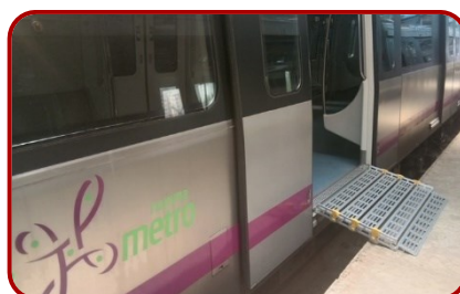
Emergency Evacuation Ramp
