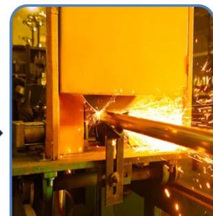
Automatic Pipe Cutting
