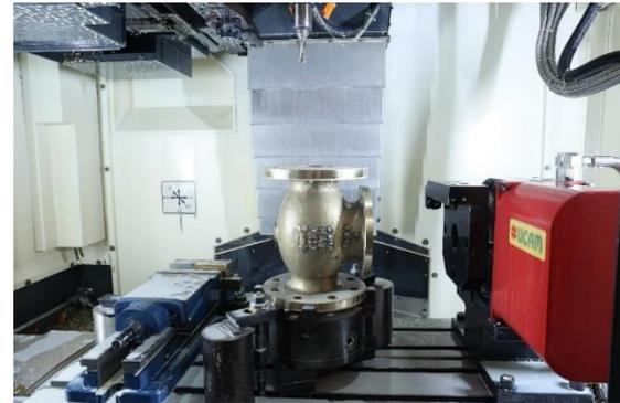
*Marine Valves Precision Machining*
