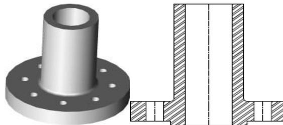
Long weld neck flanges operate when the connection pipes need to bend or go through different directions. Due to this reason, and the high pressure that occurs, long weld neck connection forging is crucial.
