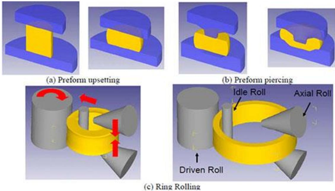
The facility is equipped with an Automated 3500T Hydraulic Blanking Press producing forged sections including crane wheels, industrial wheels, sheave wheels, gear blanks, blocks and other products. And a Radial Axial Ring Rolling Mill capable of forging Seamless rolled rings up to a diameter of 3500mm, a height of up to 750mm and a weight of up to 4 MT.
