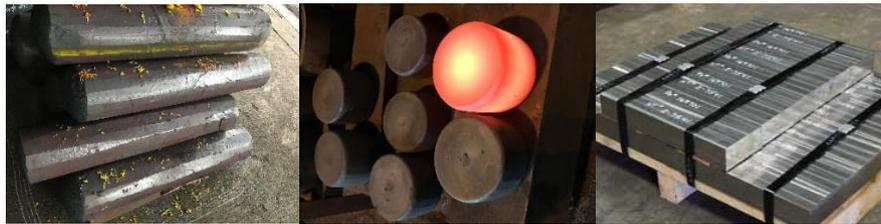
Forged alloy steel blocks are created through a manufacturing method that utilizes localized compressive force shaping processes. The process begins when steel blocks are compressed within a die and custom shaped to exact project specifications. Custom forged steel blocks are available in flat and rectangle form and are commonly used in several industries, including aerospace, food processing, chemical, oil and gas, and defense.
