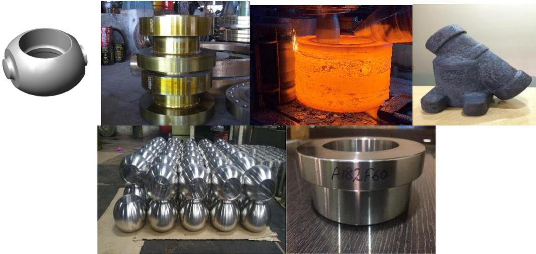
Manufacturing of valve components is done from a wide variety of materials depending on the application by the client. All Forgings such as Body, Adaptors, Balls, Stems, Trunnion Plates, Seat Rings Bonnets, and Y-Strainer Forgings are manufactured and supplied in proof machined condition.
