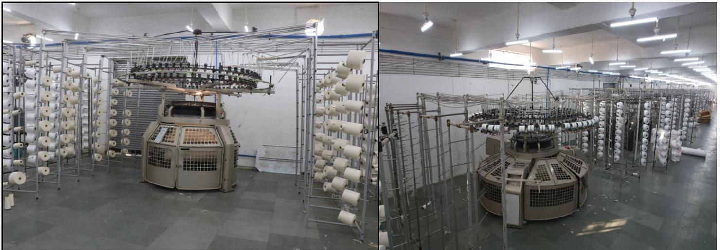
These Machines are employed in the knitting process to create the desired fabrics. Knitting machines are pieces of equipment used to knit textiles. A yarn bobbin feeds a variety of knitting techniques used in the production of the fabric. There are many diameter machines available, and each has a predetermined number of knitting sections. With a capacity utilization rate of roughly 92%, our 20 knitting machines can create 1500 tons of cloth annually.
