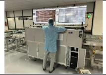
**Laminator** - It is used to join all the layers forming the module, ensuring immunity to the cell against dust, moisture, humidity, and other environmental conditions.
