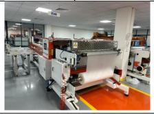
**2nd EVA Cutting machine -** Auto feeding EVA coiled material, auto cutting and punching, and laying it on the cell string.
