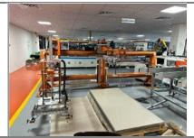
**Glass Loader** - Grasping mechanism will automatically draw glasses on the tray above the assembly line, automatically draw the separated paper into the recycle bin.
