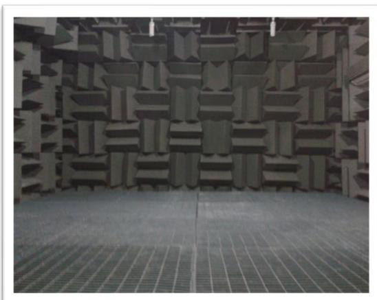
This specialized chamber is designed to replicate free field conditions above a reflective plane. At frequencies above a certain threshold, all incident sound waves on the chamber's walls and ceiling are effectively absorbed.
