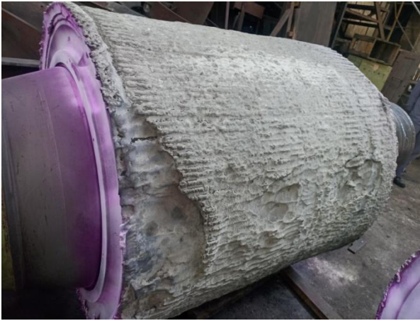
Roller Press Roll - Worn out
