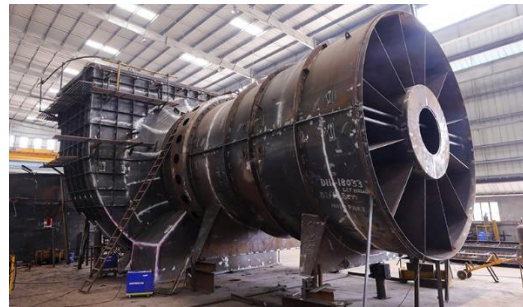
TYPE OF JOB - FGD Fans Statics Industry – Power Plant HEIGHT AND WIDTH – 9.5 Meter and width 7 meter approx. & length 20 meter approx. in assembled condition WEIGHT – 65 MT approx. in assembled condition
