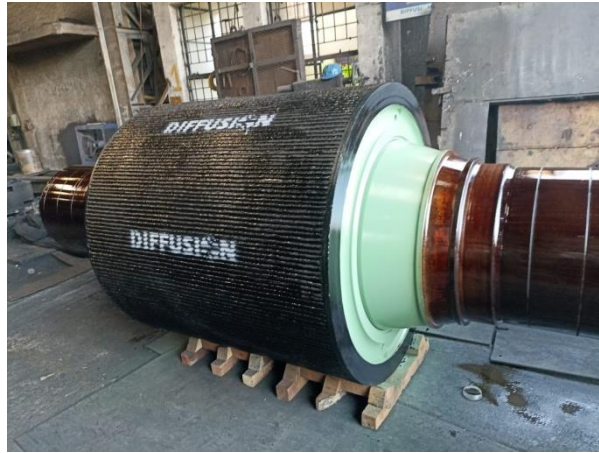
Roller Press Roll - Refurbished
