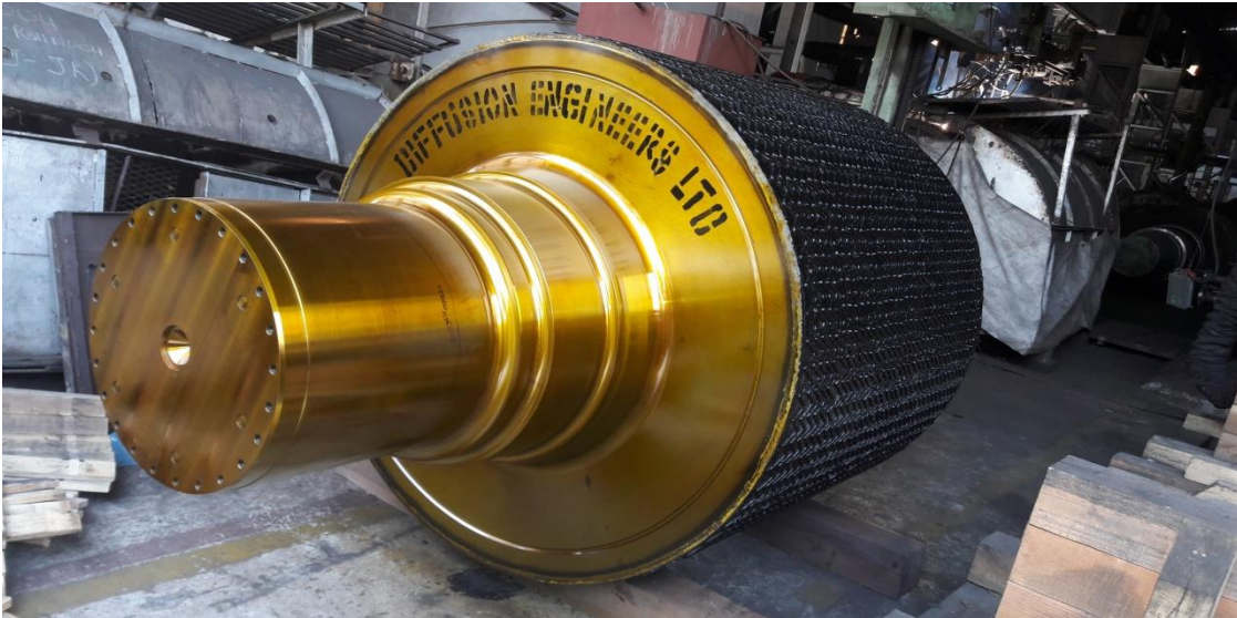
Roller Press Roll - Newly Manufactured
