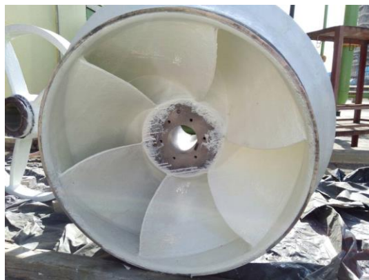
ANTI CORROSION COATING JOB
