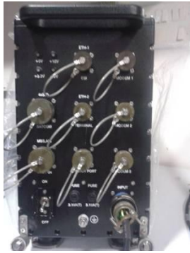
Datalink Systems 3/4 ATR •3U cPCI based •Supports Data Acquisition and Control
