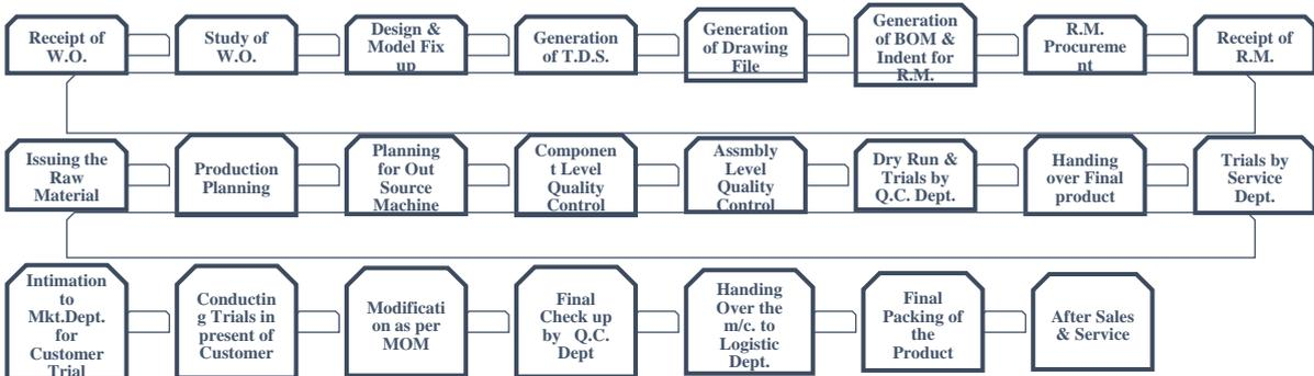
Our process for manufacturing machines starts after our marketing and sales team finalizes the machine dispatch schedule with the customer. Thereafter, the material requirement planning is calculated, following which the parts delivery schedule is sent to relevant suppliers and in-house manufacturing unit.
