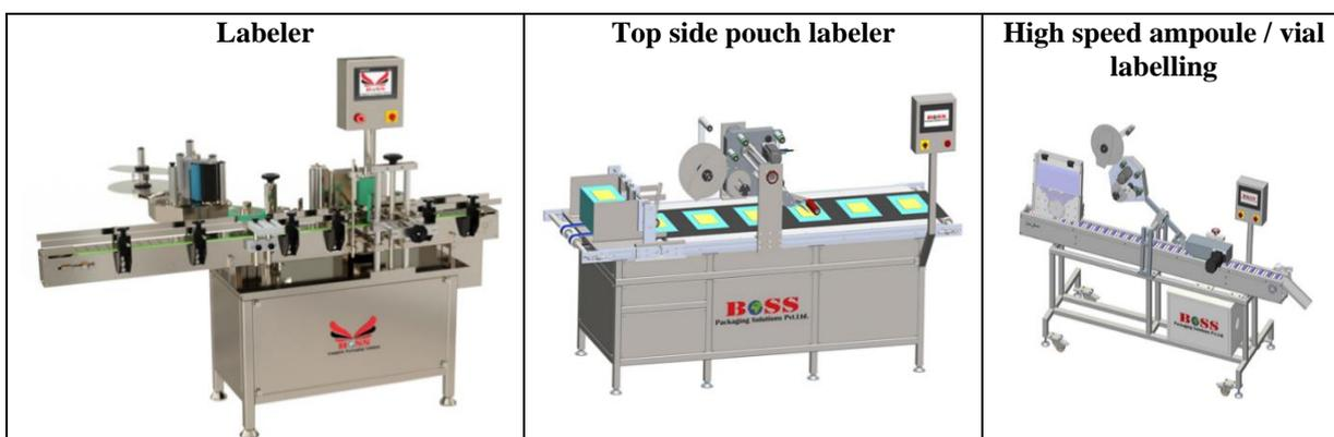
The Labelling machine is used for full/partial Labelling on different size of flat or rectangular containers. The automatic model is equipped with roller spacing device resulting in a simple operation with “No change parts required.” These machines are used in pharmaceutical / cosmetics / chemicals / agriculture and many more industries. These machines are used to paste label on the bottles / pouches / vials etc.
