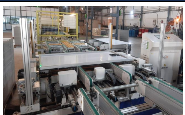
JUNCTION BOX INSTALLATION
