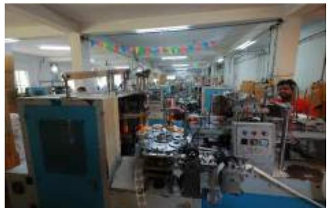
Paper Cup making machine in operation
