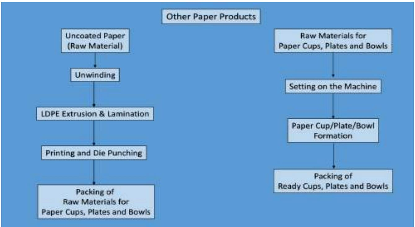
The flowchart outlines the process of manufacturing paper cups, plates, and bowls as raw materials as well as finished products.
