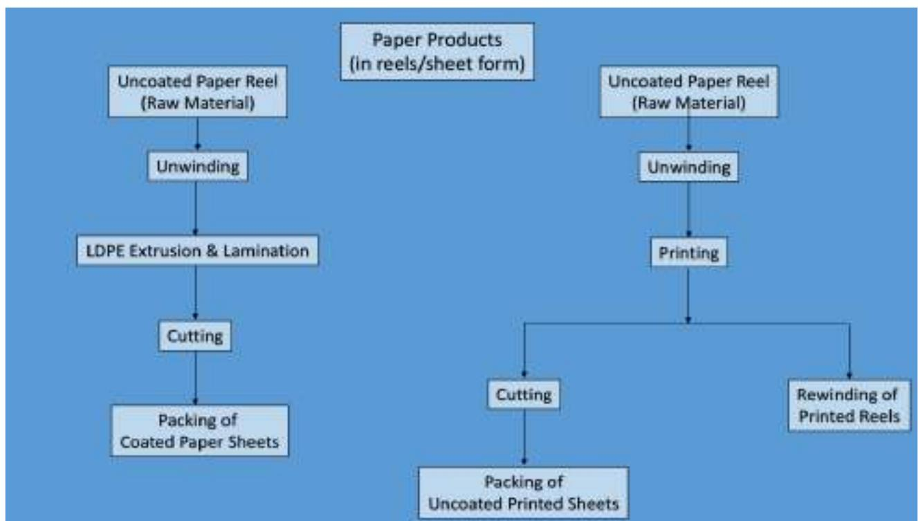
This flowchart outlines the production process for paper products, focusing on two main paths based on the treatment applied to uncoated paper reels.
