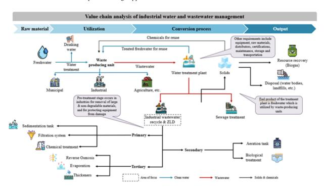
The process includes primary, secondary, and tertiary treatments to remove contaminants, with sludge generated being managed and disposed of properly. Treated effluent is safely discharged or reused within industrial processes to minimize water consumption. Advanced technologies and monitoring systems are integrated to enhance efficiency and ensure treatment quality.
