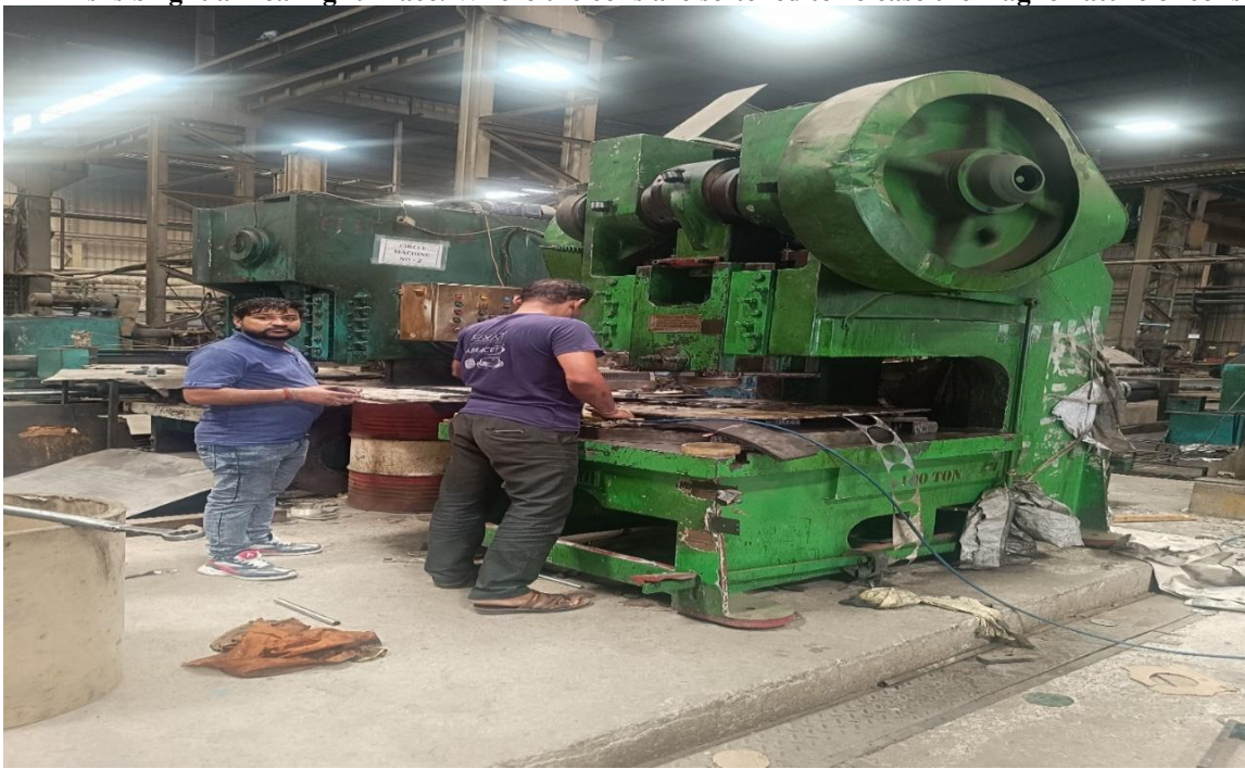
This is circle cutting machine used for cutting of circle used in utensil market.
