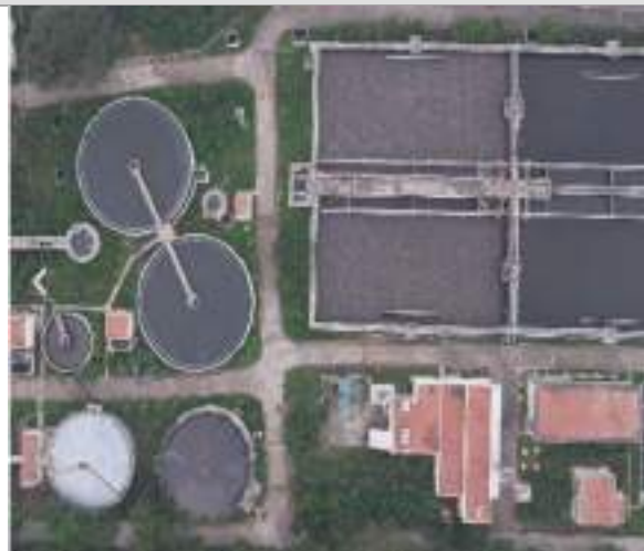
50MLD capacity Sewage Treatment Plant at Nesapakkam, Chennai with Sequential Batch Reactor (SBR) with Power Generation from bio-gas
