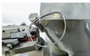
Frame Forming and Bending
