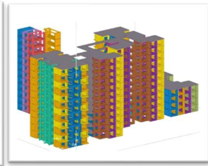
PPVC (Prefabricated Prefinished Volumetric Construction) Modules Construction
