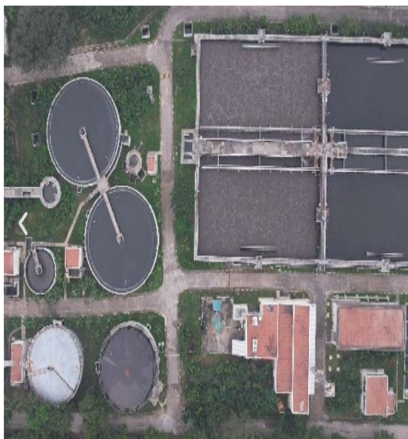
50MLD capacity Sewage Treatment Plant at Nesapakkam, Chennai with Sequential Batch Reactor (SBR) with Power Generation from bio-gas
