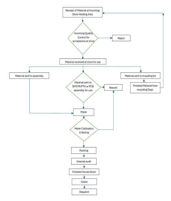
The flowchart above outlines the production and quality assurance process for energy meters, from the receipt of materials to the final dispatch to clients. Step-by-step explanation of the same is provided below:
